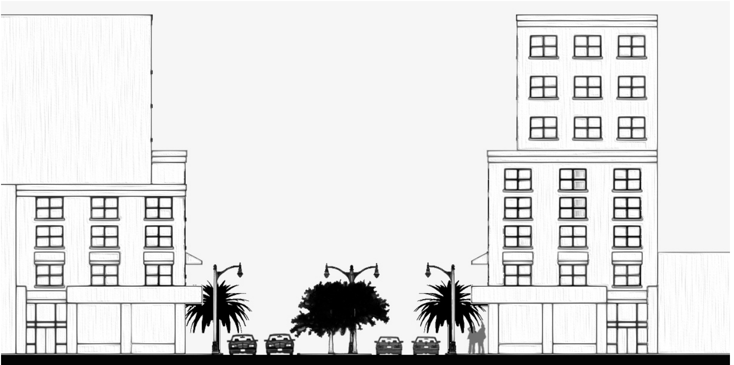
Figure 3.9: Core Street Section (SR 40, 90' ROW)
