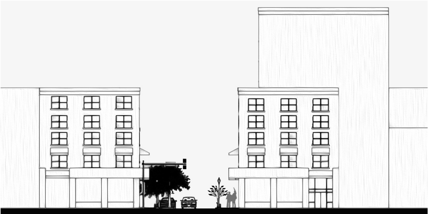
Figure 3.11: Standard Street Section (50' ROW)
